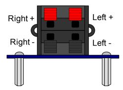
Figure 1. Stereo Full-Bridge Speaker Terminal Configuration
