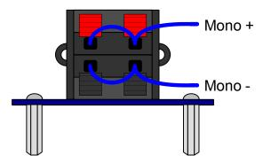
Figure 2. Mono Parallel Full-Bridge Speaker Terminal Configuration
