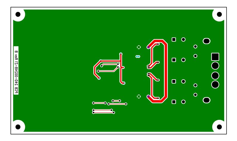
Figure 9. Bottom-side Copper Layer
