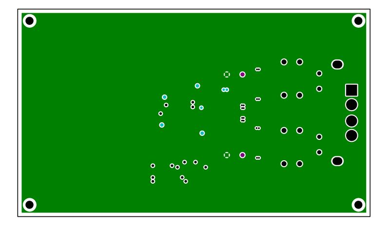
Figure 8. Inner Copper Layer 2
